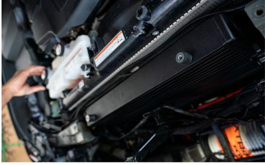
Apply rust preventative to previously drilled upper support panel—Install OEM Fasteners
