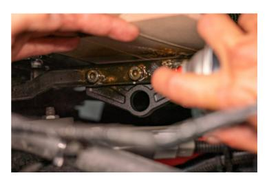
> Remove large hose clamps to coolant lines as shown below— Remove hose highlighted at both ends
