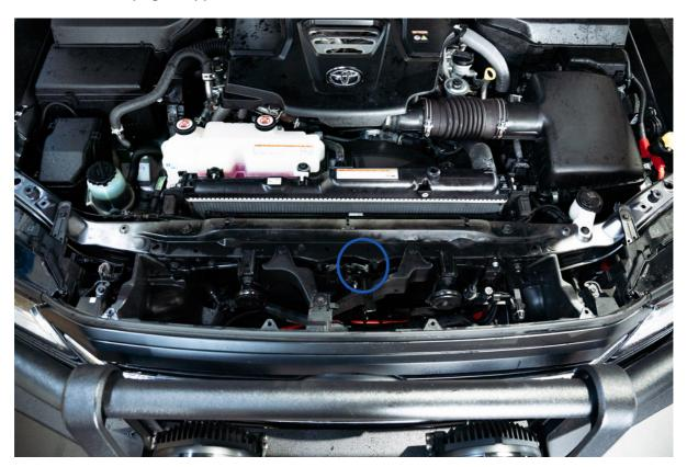
> Once fasteners are removed, allow bonnet catch to be secured out of the way
