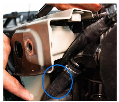
> Fit upper hose and fittings to Heat Exchanger routing as required
