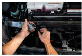
> Loosen air conditioning high pressure bracket
