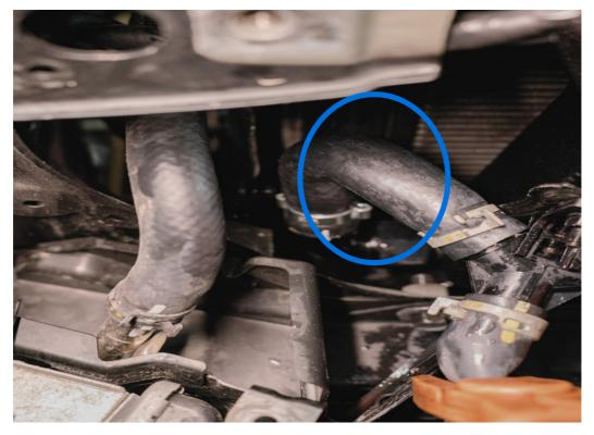
> Apply thread sealant to upper core inlet, fit 45 Degree fitting and supplied "J" hose, fit clamps as required.
