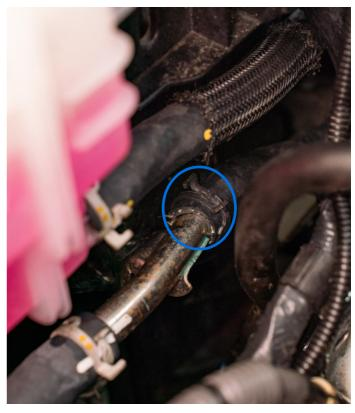
> Locate supplied bleed bung, apply thread sealant to the bung. Note - Do NOT install bung until coolant has been refilled, this is in preparation for the next step
