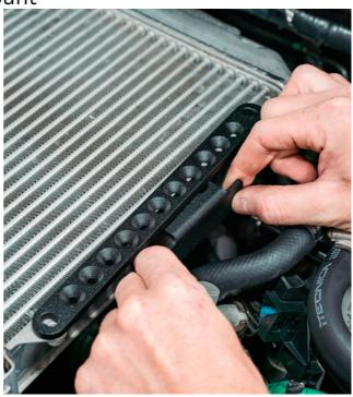
Fit adjustable bracket and locate a suitable position for relays to allow fitment Apply counter sunk fasteners to bracket
