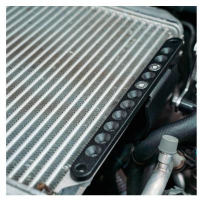
Install adjustable bracket as spacer on passenger side (LHS) Install low fan mounting plate
