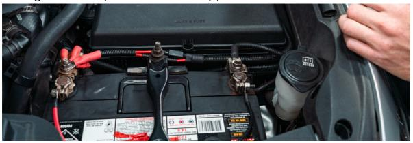
> Turn vehicle ignition on till dash light illuminate - Fans should start to cycle. Turn vehicle ignition off - Fans should cycle off.
